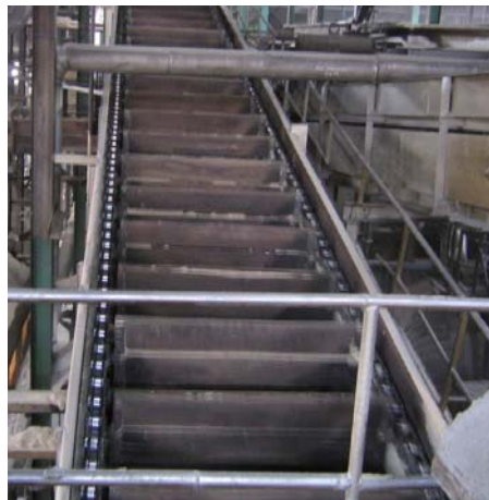
Bagasse carrier SS2184 A42+2C SS1796 A42+2C
